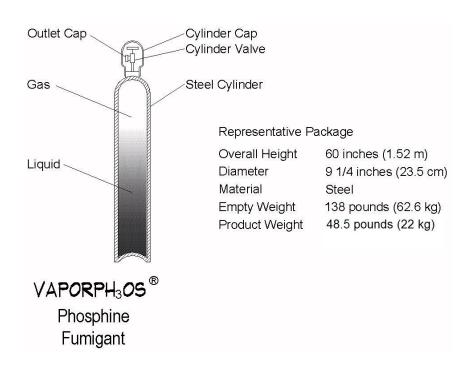
The product flows to the blending equipment through the cylinder outlet valve. As gas is withdrawn from
